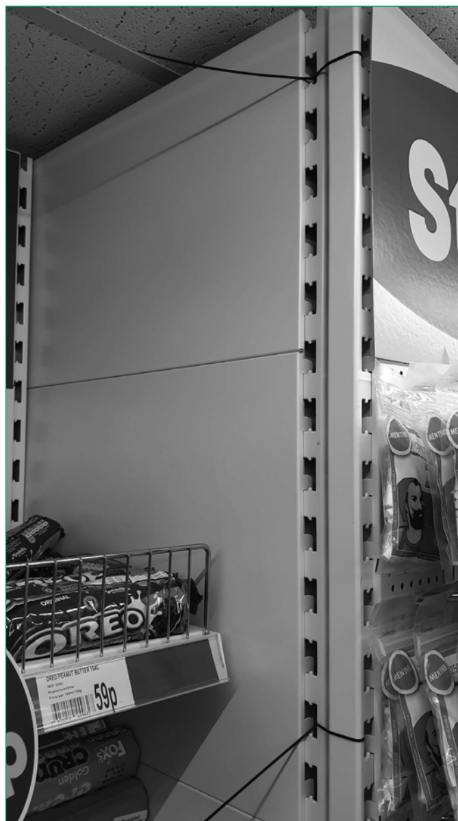
Uprights connected with zip ties. Definitely not the correct, strong solution.
