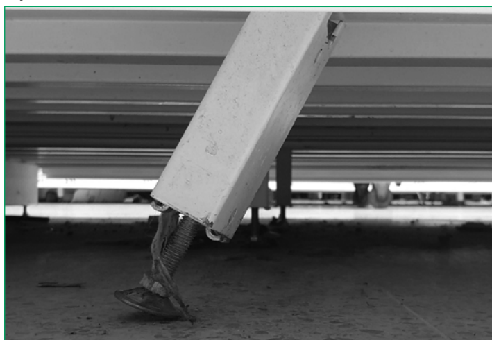
The leveller on this gondola unit was incorrectly displaced during use in a busy store. This could easily cause failure under load. Regular checks should be carried out.
