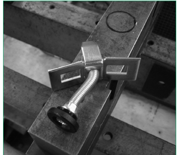
A foot which has completely failed due to excess load.
